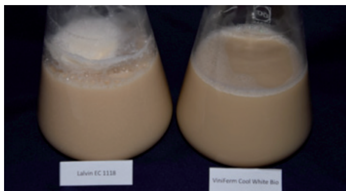
Picture 1: Comparison of foam production between a conventional (Lalvin EC1118) and an organic, emulsifier-free (ViniFerm Cool White Bio) yeast strain.
